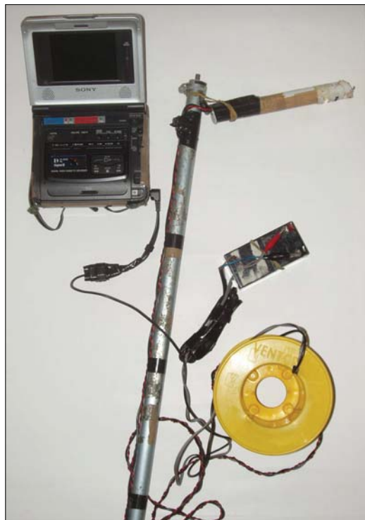
Fig. 4. The full system showing the camera, aluminium pole, battery, video recorder and cables.
