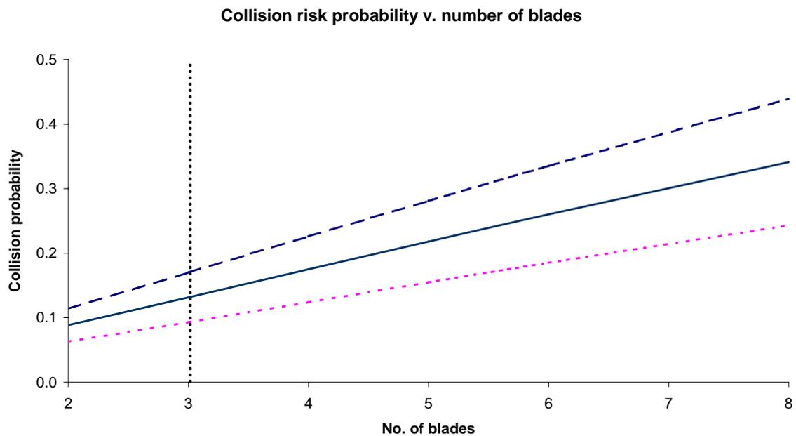
**Figure 4** Effects on collision risk of variations in parameters used in the collision risk model (based on the SNHWB spreadsheet). The upper dashed line represents the 'upwind' scenario, the lower dotted line the 'downwind' scenario and the solid middle line the average between the two. In each case, original values (Fig. 1) remain constant apart from the parameter in question. Original parameter values are denoted by a vertical line.
